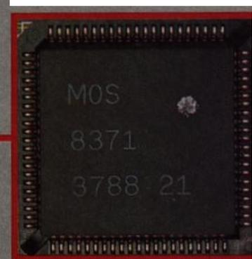
The Agnus chip. If the one on your board is numbered 8370 or 8371 it needs to be replaced with the newer 8372A chip so that you can access up to 1Mb of Chip RAM.
